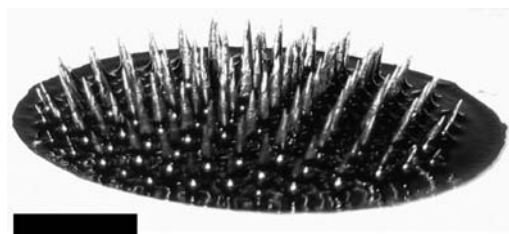
FIGURE 5. Photograph of a concentrated solution of CoFe 2 O 4 nanoparticles in hexane placed on top of a permanent magnet (~0.4 T). Scale bar is 1 cm.
